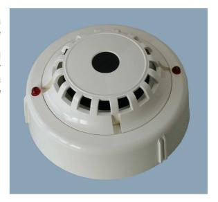
The MHG 231 detector is installed at places where occurrence and concentration of smoke is assumed. The detector is responsive to visible and invisible smoke particles (aerosols) – on the principles of detection of scattered infrared radiation.
