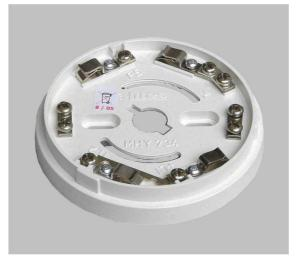
The MHY 734 Base is powered with AC voltage 24V (two pole terminal). Power supply voltage is streamlined and stabilized. In the case of activation of fire detector to alarm state it is switched on alarm rellay in the base. Independent changeover contact of relay (wired to the three-pole terminal) can be used to control e.g. fire closure. The base is adapted from the base MHY 734
